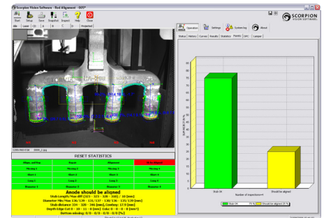
Inspection result with measured values and Pareto graph.
