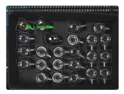
3D Bin picking in a box of valves. Scorpion sends the valve positions to the robot.
