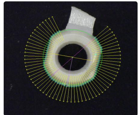
*The CircleGauger calculates ovality, the minimum, maximum and mean radius and visualizes the minimum and maximum radius points.*
