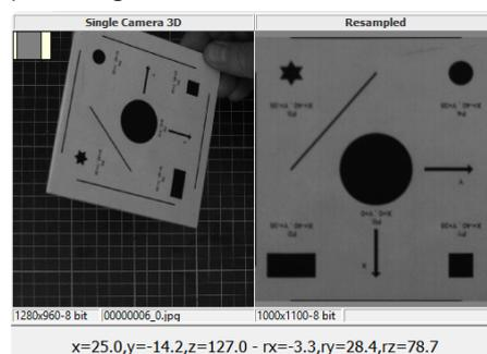
*The image is resampled based on the single camera 3D pose*
