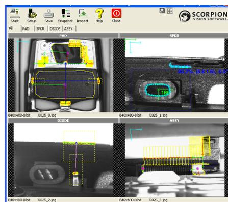
A four camera Scorpion system doing assembly verification on a mobile phone.
