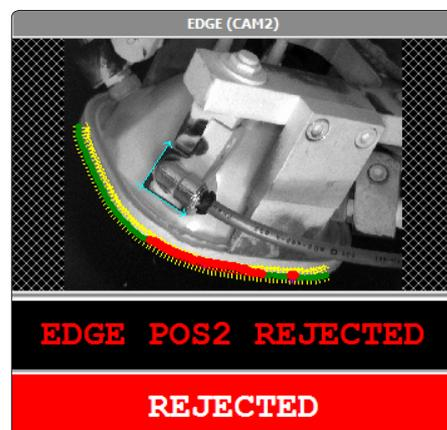
A two camera and six images solution detecting minor cracks and edge defects on a automotive plastic part.
