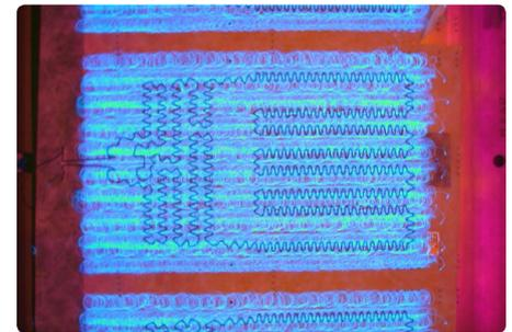
*Glue distribution is measured using colour identification.*
