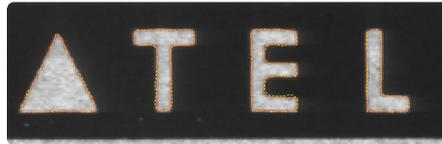
PolygonEdgeFaults2 verifies the edge of the print. The model are translated, rotated and scaled using PolygonMatch technology before edge verification.
