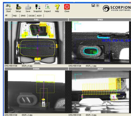
*A four camera Scorpion system doing assembly verification on a mobile phone.*
