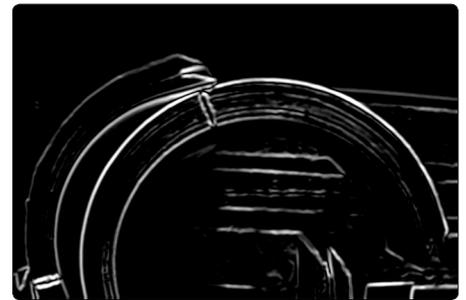
*The image is processed with Image Filter with the following features: Dynamic skew removal, Median Filtering, Sobel Filter and Contrast adjustment.*
