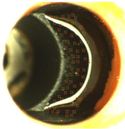
*ColorMatcher™ detects glue coverage on a pressure sensor.*
