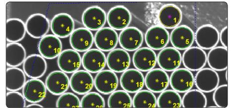
Blob4 sorts results into row and columns. The collection of sorted pipes are shown. A robot will pick the uppermost pipe until the bin is empty.
