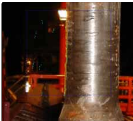
LineFinder finds the edge of a drill pipe based on changes in color.
