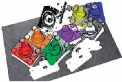
3DMaMA locates seven parts located in 1 second in an occluded scene
