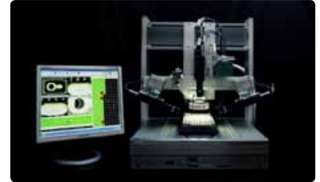
Sony desktop robot, firewire cameras and Scorpion Vision Software working together.
