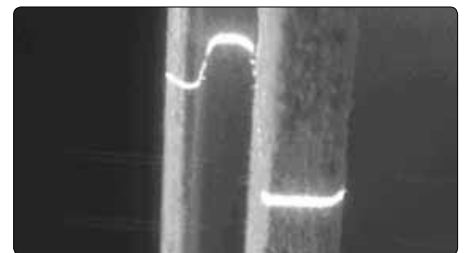
The example above shows the laser profile generated by the edge of a Medium Density Particle board.
