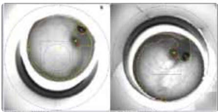
Measuring the intensity of pixels within a circular region determines whether eggs are dead or damaged. Should four dark areas assumed to be eyes be present, the egg likely contains twins as seen above.
