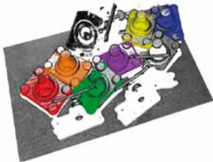
3DMaMA locates seven parts located in 1 second in an occluded scene
