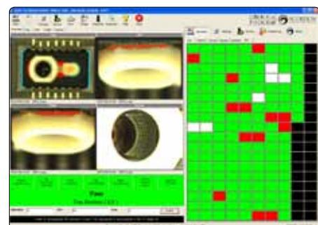
*Clicking in the matrix on the screen moves the robot in position and re-inspects sensor.*
