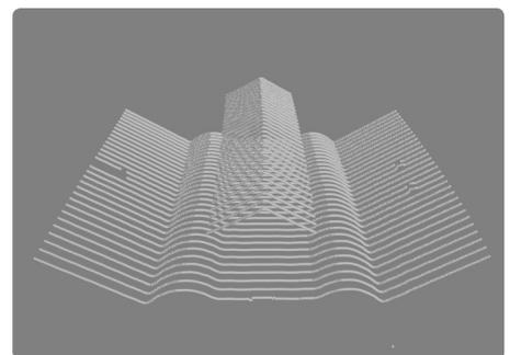
*Thickness measurement of a knife*
