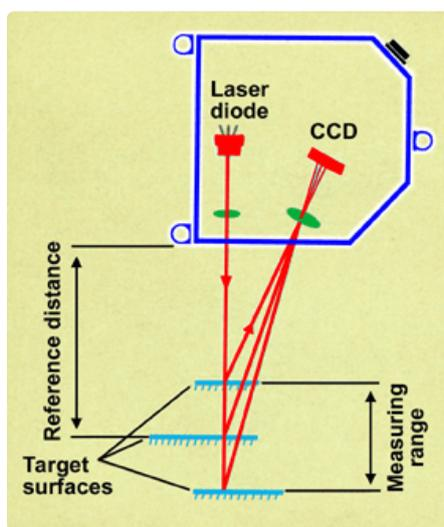
*The concept of 3D Laser Triangulation*
