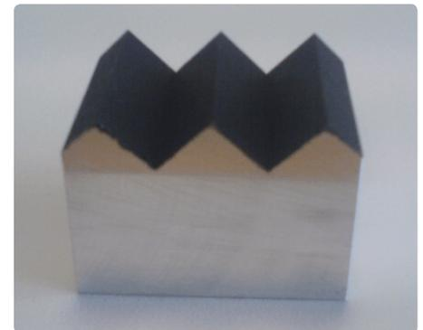
*Saw tooth shaped calibration object*
