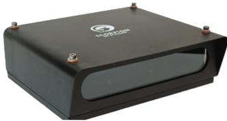
By mounting the system on a robot, it is possible to model the complete surface of any product.
