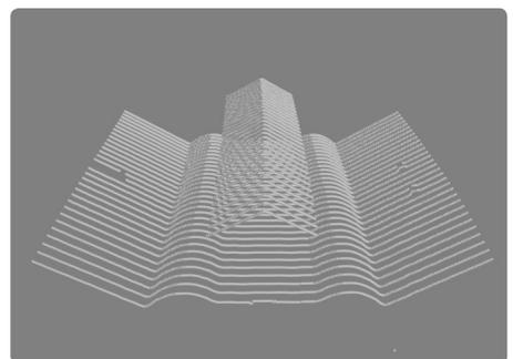
*Thickness measurement of a knife*
