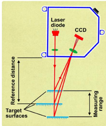
*The concept of 3D Laser Triangulation*
