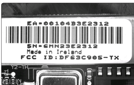
The 1D Barcode is used to identify the circuit board.
