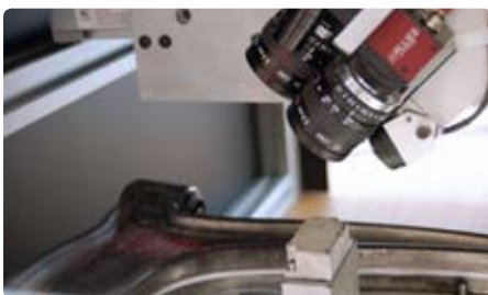
Image 4, Matrix laser light source generating bright dots on an automotive part
