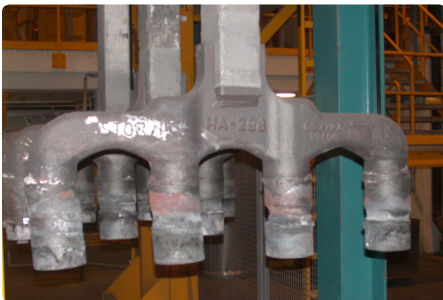
Anode ready for stub alignment
