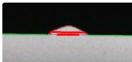
All wafer edges are checked for defects, missing material and glue residues.
