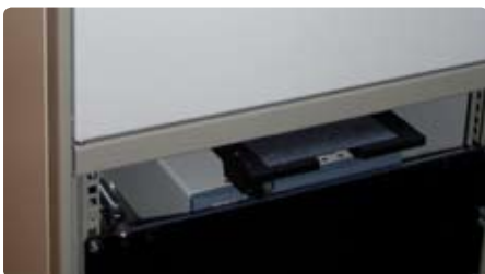
Wafer placed in cabinet fixture. The desktop robot positions the wafer under the cameras and grid.
