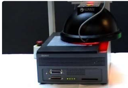
Robot scanner detecting wafer contamination.
